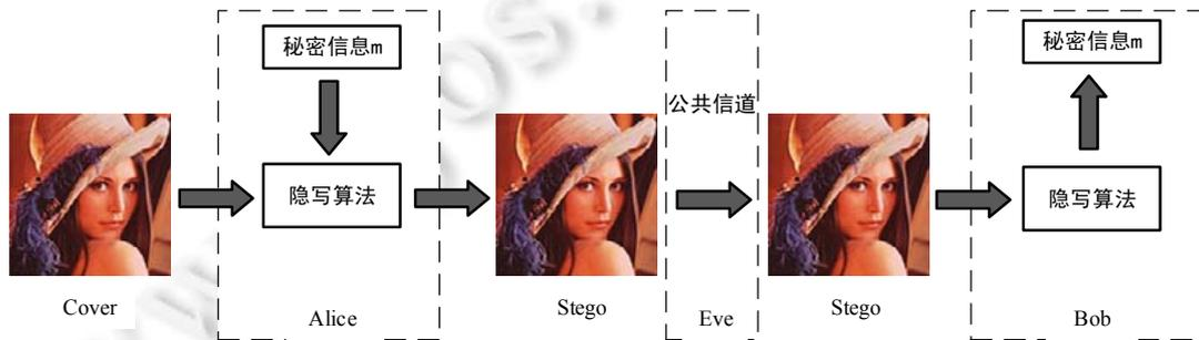
Fig.1 General process of steganography
