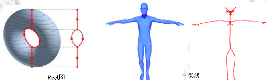
Fig.2 Diagram of Reeb graph and skeleton with different shapes
