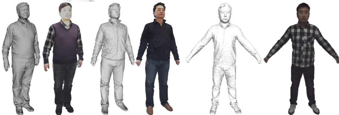
Fig.4 3D full-body results for typical adults. In each case, left: reconstructed geometric mesh, right: textured model. Personal details, such as faces, cloth wrinkles, and hairstyle, are well captured
