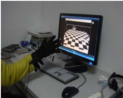
Fig.1 The operator is interacting with the computer with data glove and position tracker on her hand
