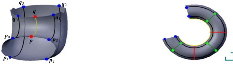
(a) Connect the corresponding vertex pairs directly (a) 直接连接对应顶点 (b) Connect the corresponding vertex pair through the reference cycle (b) 通过参考环连接对应顶点
