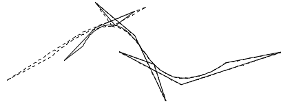
Fig.2 DP-NTP spline curve of degree 4 and its control polygon
