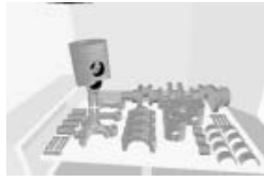
Fig.7 Recognized 'hole-hole align' semantics and taken the mate constraint of end faces of two holes as motion guidance constraint 图 7 识别出“孔-孔对齐”语义,将孔端面贴合约束作为运动引导约束
