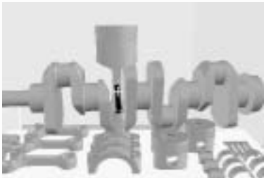
Fig.10 The recognized 'bolt-hole-nut joint' semantics and taken the align constraint of centerlines of bolt and hole as motion guidance constraint 图 10 识别出“螺栓-孔-螺母联接”语义,将螺栓与孔轴线对齐约束作为运动引导约束
