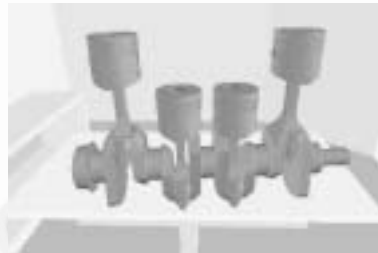
Fig.11 Final assembly of piston and connecting rod component of automotive engine 图 11 装配好的汽车发动机的活塞-连杆部件
