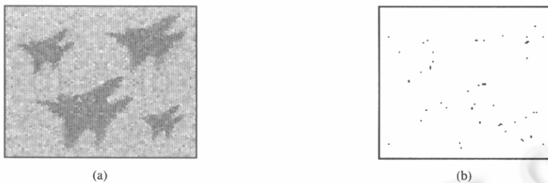
Fig. 9 The result of corner detection for gray image by using operator Cor_z
