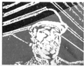
(a) Binary image of absolute difference without motion compensation
