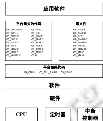
Fig.2 Code structure of \mu\text{C}/\text{OS-II}
