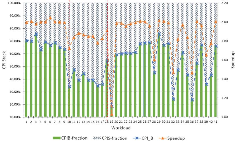
Fig.3 The correlation between the CPI Stack and the application speedup
