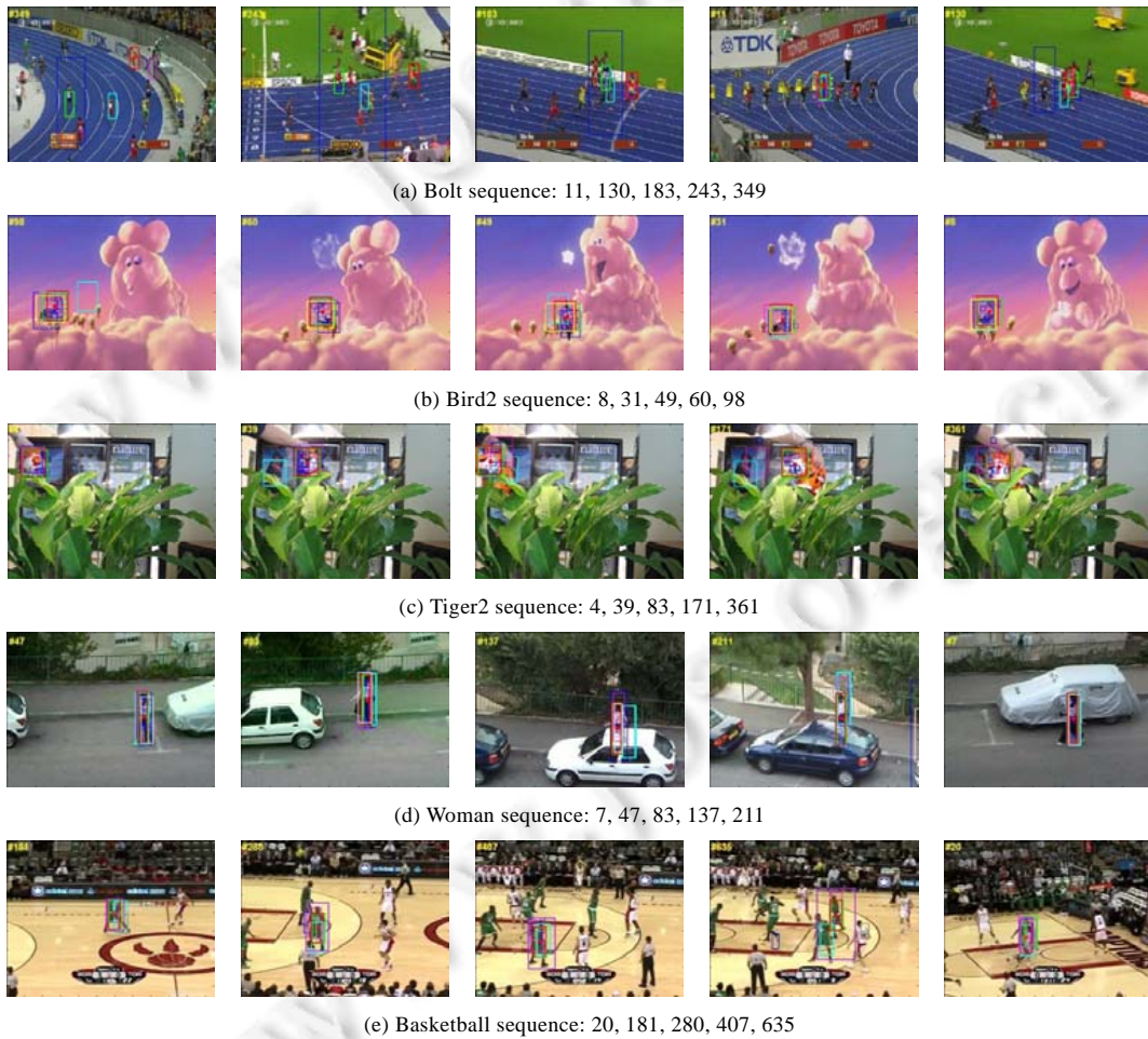
Fig.6 Comparison of some tracking results on different sequences
