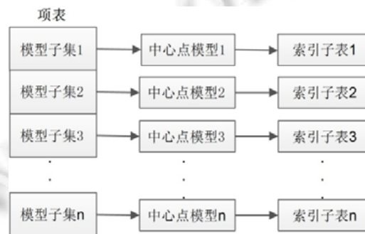
Fig.4 Diagram of data structure of physical inversion table
