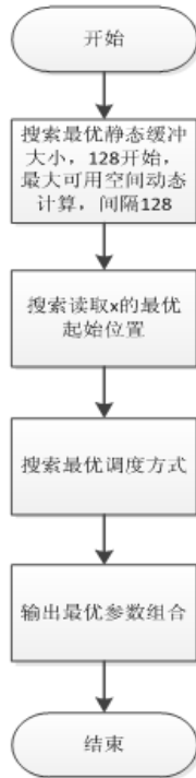
Fig.5 The flowchart of search of optimal parameter
