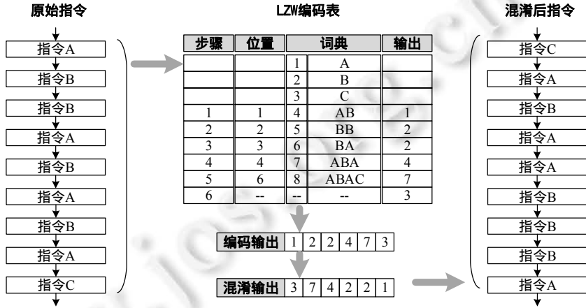
Fig.6 LZW encoding process during obfuscation
