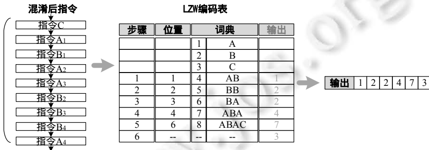
Fig.9 Process of LZW decoding algorithm for some sequence of instructions
