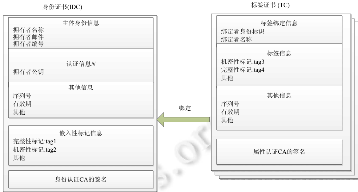
Fig.9 Format of identity certificate and tag certificate 图 9 身份证书与标签证书格式
