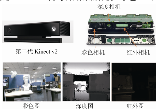
Fig.1 Hardware and raw data of Kinect v2
