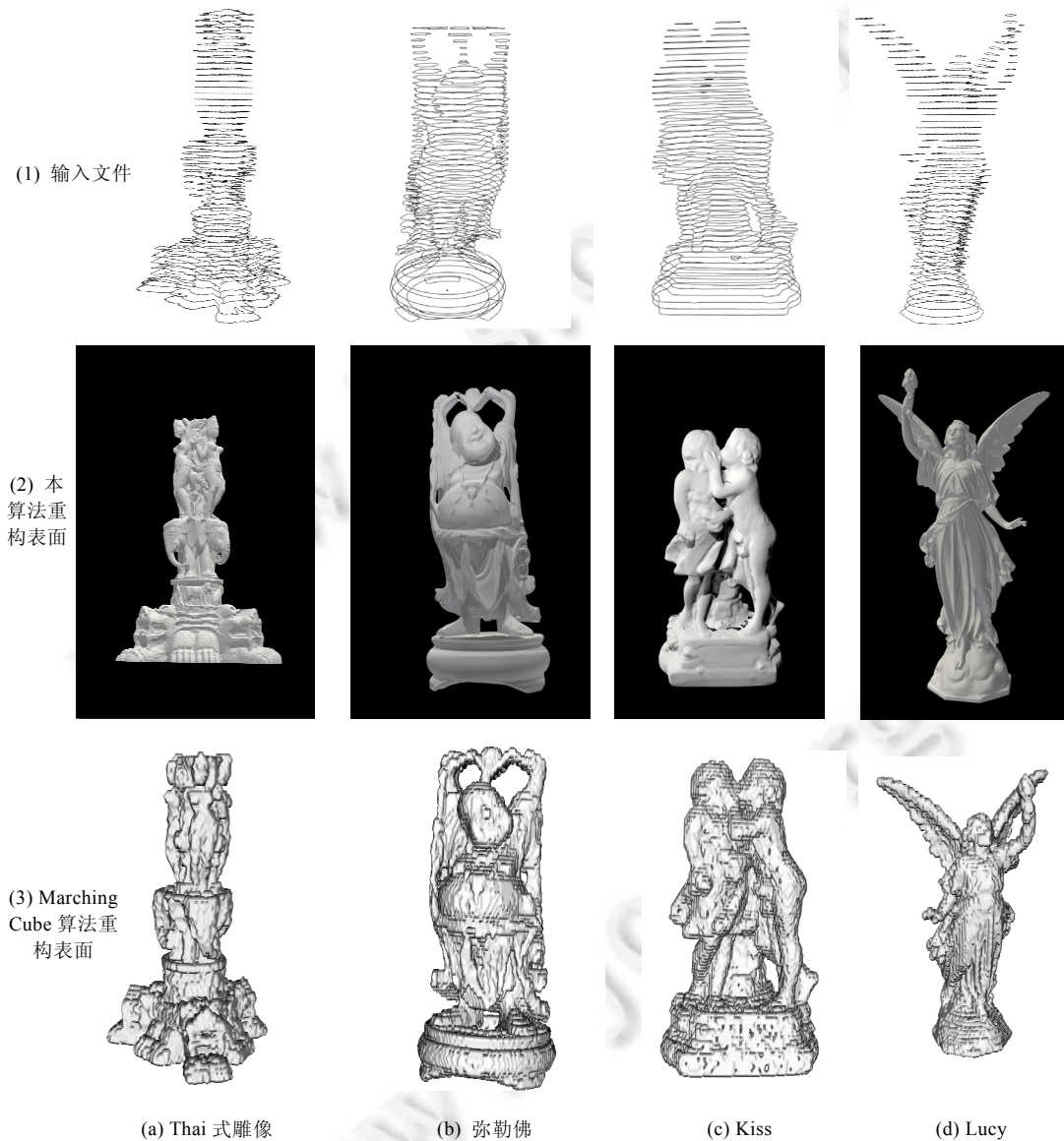
Fig.12 The comparison between our method and Marching Cube method
