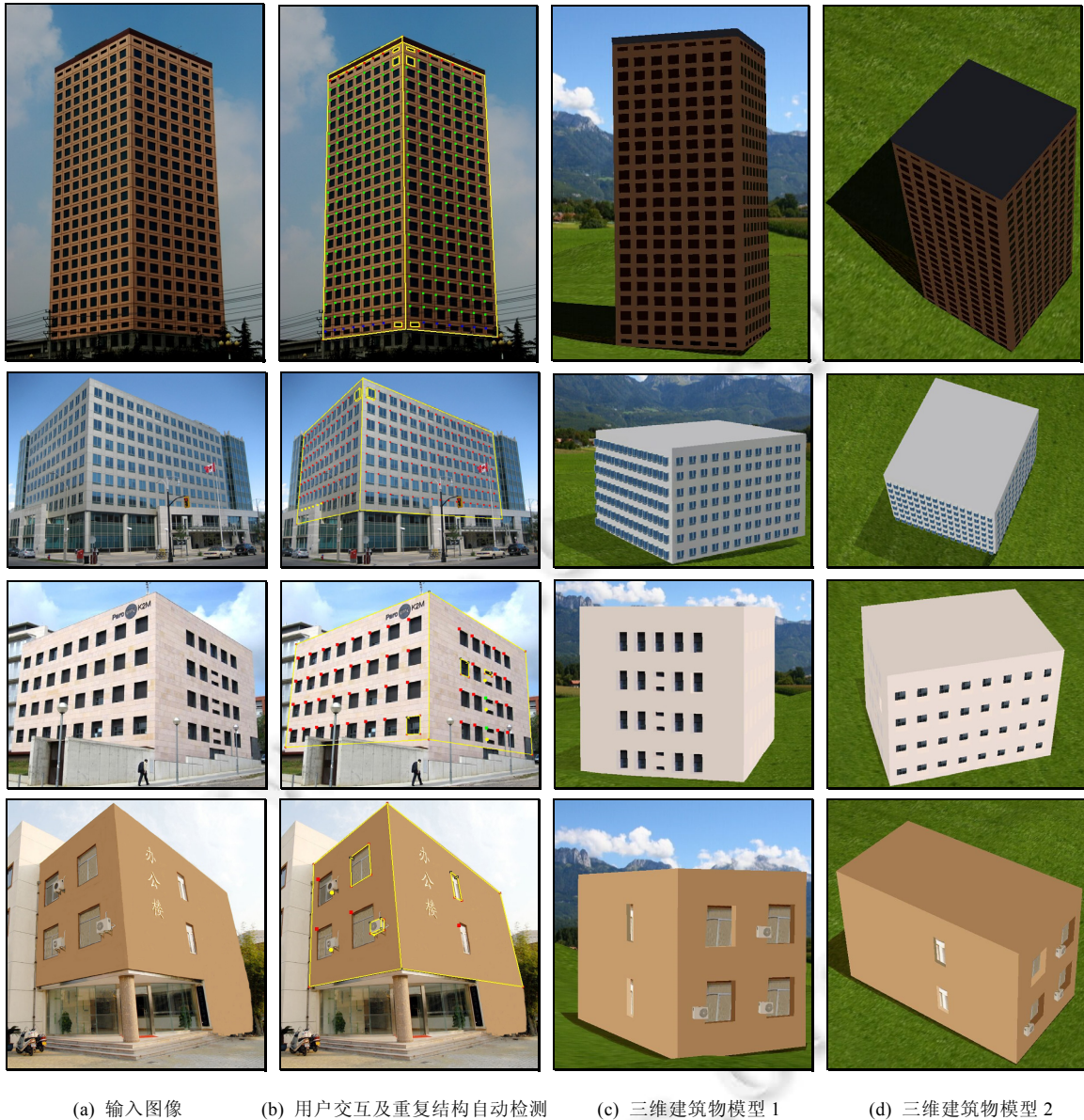
Fig.10 3D architecture modeling based on repetitive structure detection
