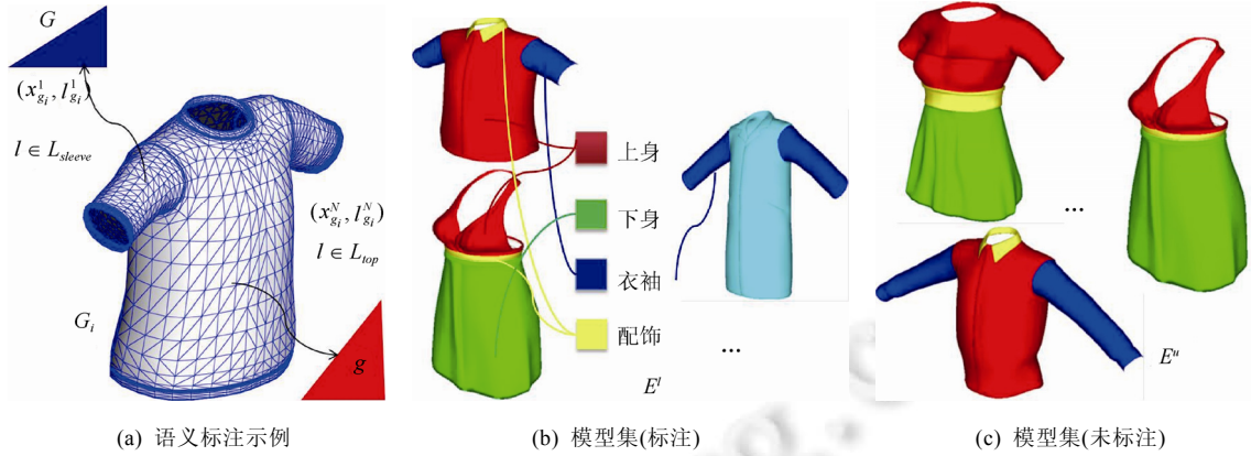
Fig.2 Example of semantic labeling for 3D garments, the training meshes includes labeled and unlabeled garment 图 2 三维服装模型语义标注示例,标注过的以及未标注的服装网格模型集作为训练集
