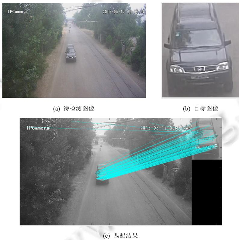
Fig.2 Target matching using SIFT feature
