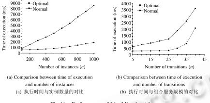
Fig.11 Performance of LiveMig algorithm 图 11 LiveMig 算法的性能
