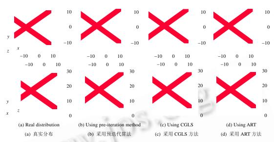
Fig.3 Top view and side view pictures for the real distribution of double fluorescent targets and the reconstructed results using different inversion methods
