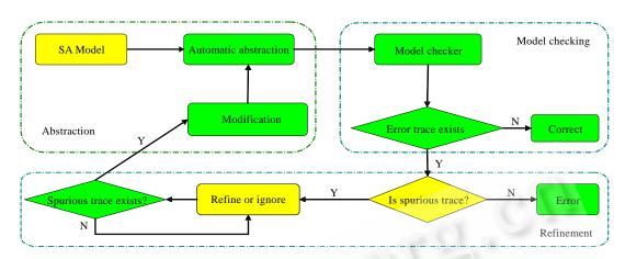
Fig.5 The process of negotiation-enabled model checking
