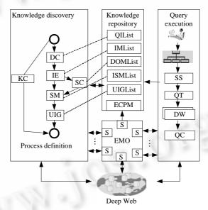
Fig.2 Dynamic software architecture for large-scale deep Web integration 图 2 大规模 Deep Web 集成动态软件体系结构
