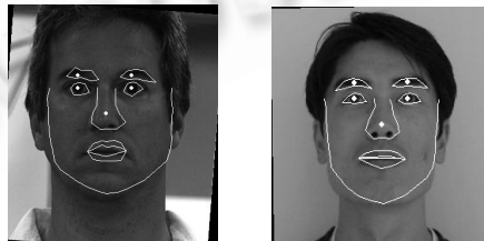
Fig.8 The failure examples of facial landmarks labelling 图8 面部特征标定失败的样例
