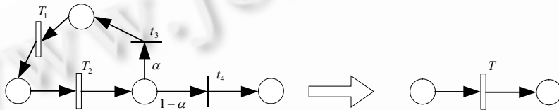
Fig.5 Iteration subnet and its simplification
