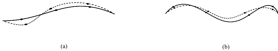
Fig.5 Shape modification of Bézier curve with multiple target points
