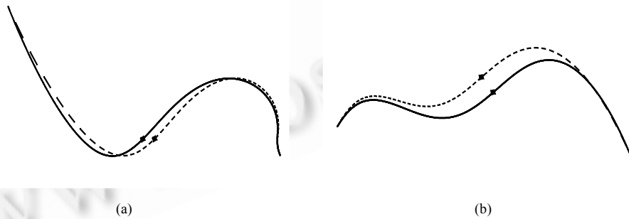
Fig.4 Shape modification of Bézier curve with single target point
