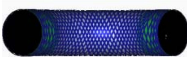
Fig.5 A filament winding with \mu = 0.2 , \alpha_0 = 78^\circ , w = 10\text{mm}
