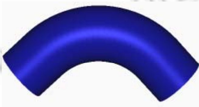
Fig.7 A finished wound elbow with \mu = 0.2 , \alpha_0 = 76^\circ , w = 10\text{mm}
