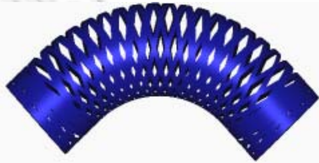
Fig.6 A winding pattern with \mu = 0.2 , \alpha_0 = 78^\circ , w = 15\text{mm} without mandrel
