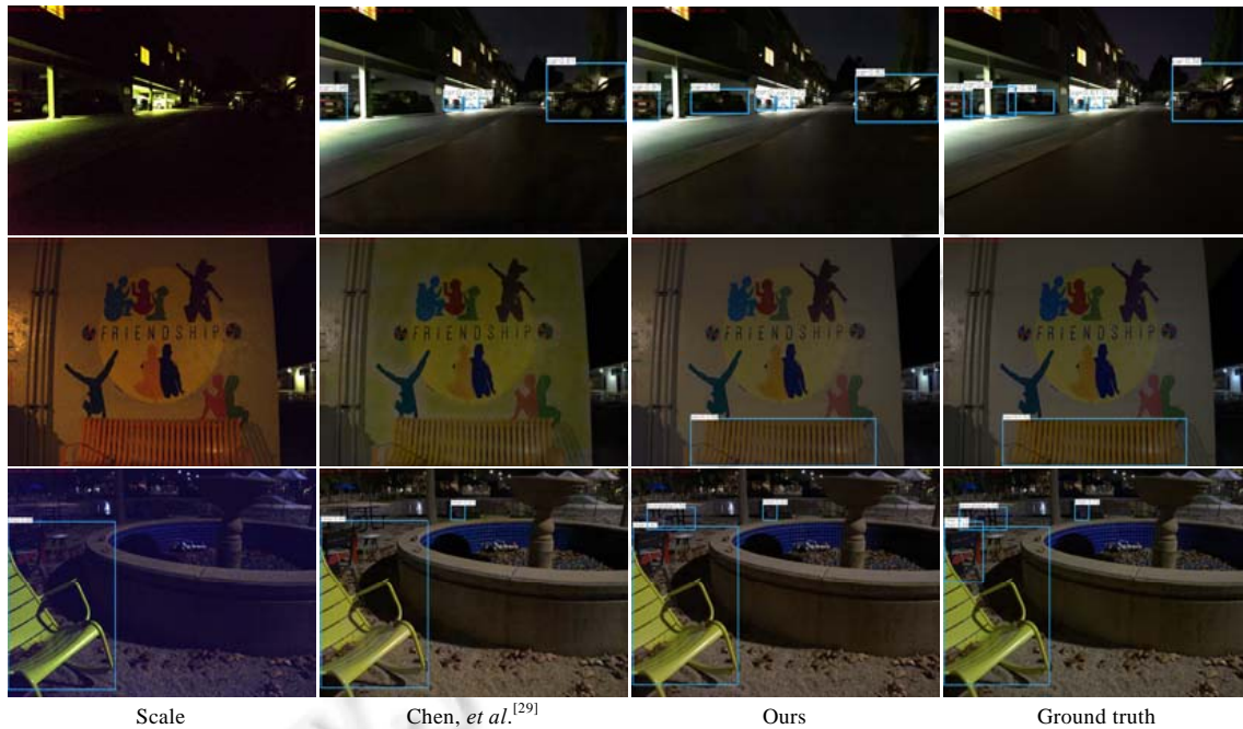
Fig.5 Object detection results of low-light images restored by different methods on YOLOv3 (Please zoom in to the detailed recognition confidence)
