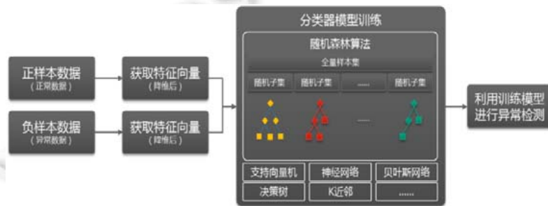
Fig.13 Supervised graph anomaly detection algorithm framework
