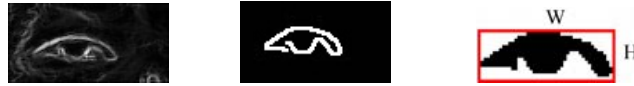
Fig.6 Edge detection results and eye aspect ratio R=H/W , where R \in (0, +\infty)
