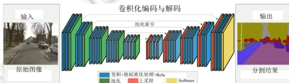
Fig.7 Framework for SegNet-Basic<sup>[60]</sup>
