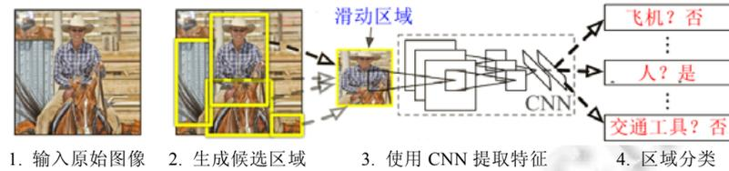
Fig.3 Workflow for RCNN<sup>[12]</sup>
