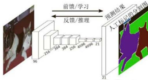
Fig.5 Framework for FCN<sup>[23]</sup>图 5 FCN 框架结构<sup>[23]</sup>**Table 2** Comparison of fully-supervised image semantic segmentation algorithm based on pixel classification**表 2** 基于像素分类的全监督学习图像语义分割方法对比
