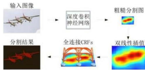
Fig.6 General framework for DeepLab<sup>[25]</sup>
