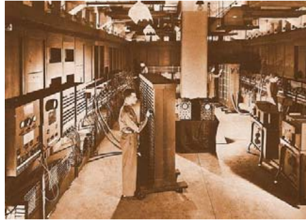
Fig.1 Programming ENIAC by a combination of plugboard wiring and portable function tables [7]
