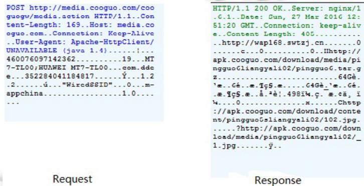
Fig.3 Request and response data of Kuguo SDK
