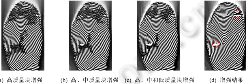
Fig.9 Fingerprint enhancement based on quality grading scheme and the compsite window strategy by using orientation Gauss band-pass filter
