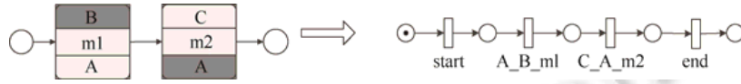
Fig.9 A choreography violating the basic rule of choreography activity sequencing and the corresponding WF-net
