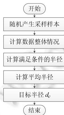
Fig.3 Flow diagram of calculating radius d_c
