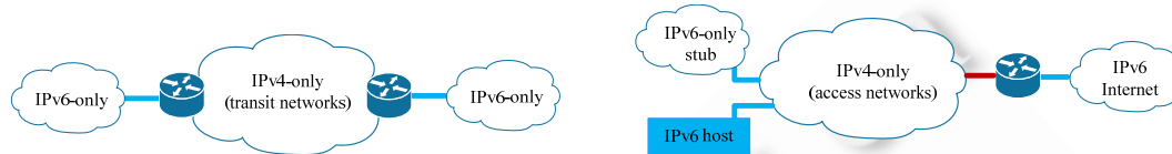
Fig.5 IPv6-over-IPv4 transition scenarios
