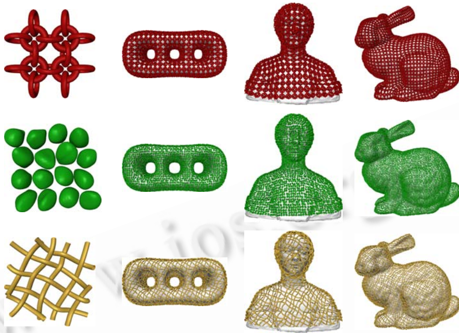
Fig.6 Results of geometric texture mapping. Left: Geometric textures. Right 3 columns: Three mapping results 图 6 几何纹理映射的结果.左边一栏是几何纹理.右边三栏是映射的结果
