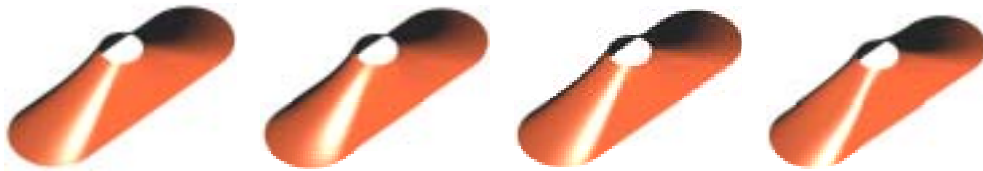
Fig.8 Control the whole surface through modifying the shape of curves in the connected position 图 8 通过修改拼接曲线的形状来控制整个曲面
