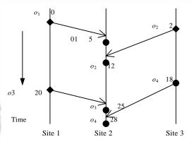
Fig.3  $\delta_1^2 = 5$ ,  $\delta_3^2 = 10$ , operation  $o_1$  and  $o_3$  are issued on object x at site 1, whereas  $o_2$  and  $o_4$  are issued on y at site 2
