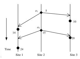
Fig. 2 Delay time from site 2 to site 1 is 9, whereas the delay time from site 2 to site 3 is only 5
