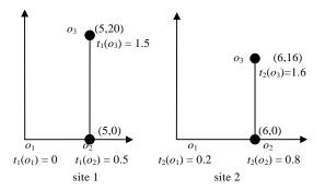
Fig.1 Example of an inconsistency problem in object with continuous media. Site 1 issues three operations at time 0, 0.5 and 1.5, respectively. The communication delay for operations are 0.2, 0.3 and 0.1. The final position at site 1 is (5, 20) and the position after executing  $o_3$  at site 2 is (6,16).
