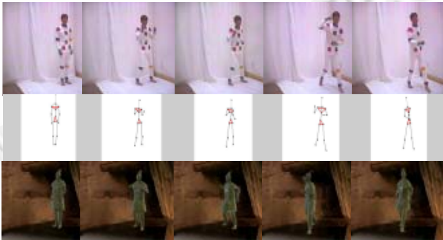
Fig.5 Boxing clip (the first row is original video, the middle row is stick model, the last row is QinYong animation)
