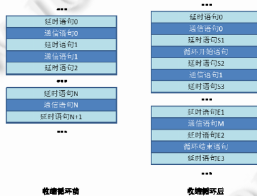
Fig.2 Adding delay statements after repeat-compression
