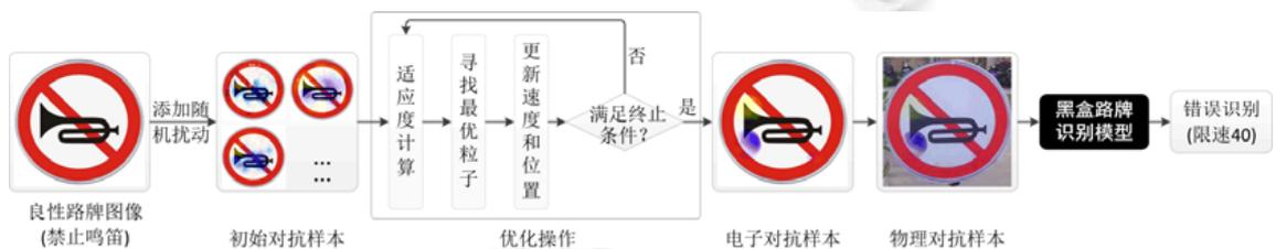
Fig.2 Framework of black-box physical attack against road sign recognition model via PSO
