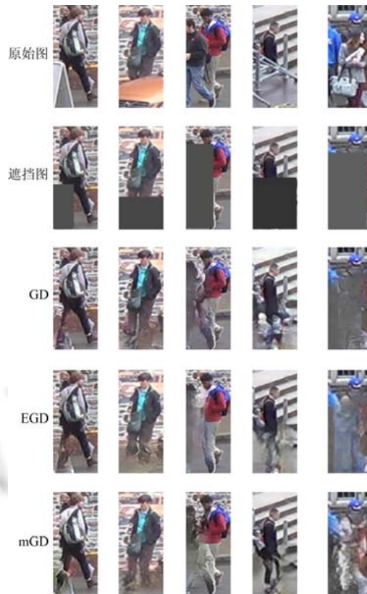
Fig.4 The de-occluded images obtained by different methods on the occluded query set of Duke MTMC-reID
