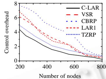
Fig.15 Control overhead vs. number of node
