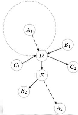
Fig.1 Improper control of the RREQs
