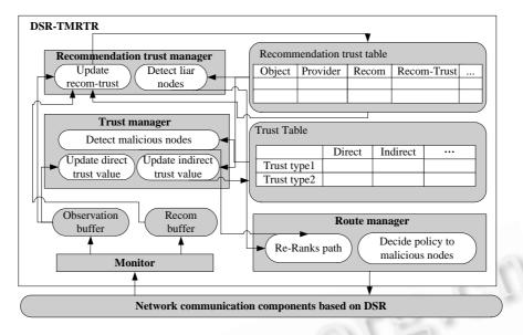
Fig.1 Components of DSR-TMRTR
