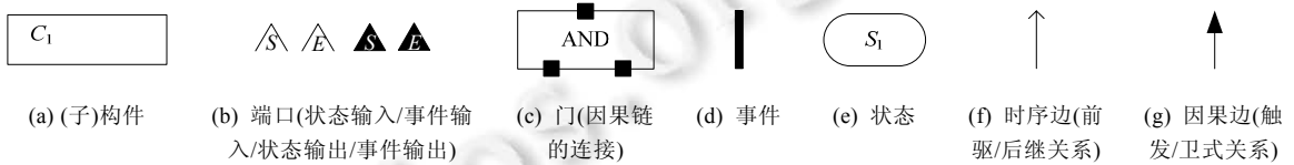
Fig.1 Main modeling elements of SEFT
